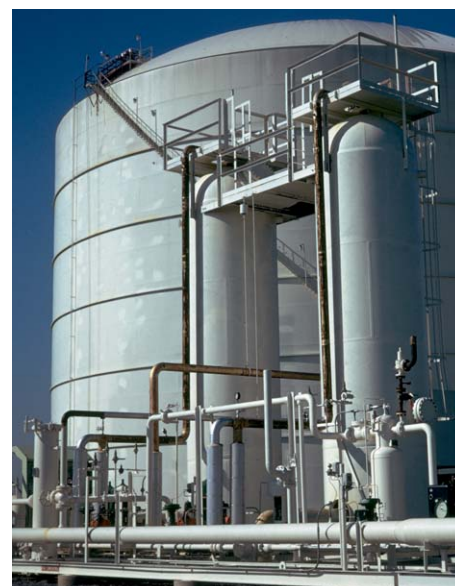
Multiple bed adsorption for H 2 O and CO 2 removal from natural gas before methane liquification.
